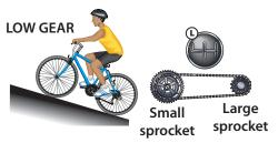
Shifting Gears A car's transmission works just like the gears in a bicycle. High gear combines the larger crank sprocket with the smallest sprocket at the rear wheel.
